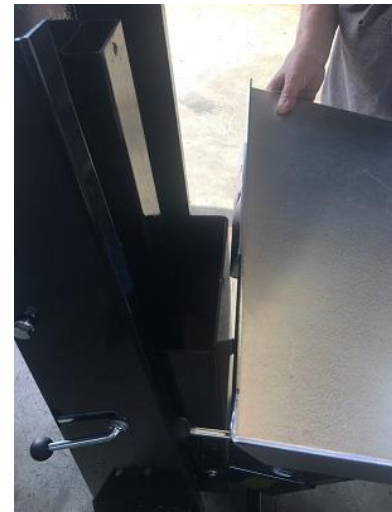
Set the table back on the rest on the column
