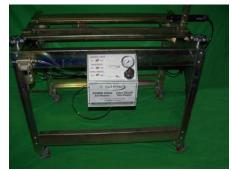
rollers to the support frame and start the stone drive, spin motor and linear actuator, make minor adjustments to align the stone to the reel and leave the PowerEdge II to take care of the rest. After just a few minutes, the edges of the reel blades will be "factory fresh" with a sharp cutting edge offering maximum performance from the reel mower.
