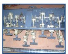
The unique design of the **CRANK ASSEMBLY** with perfectly timed offsets between each connecting arm assembly maintains balance <u>without</u> the need of counter weights. The connecting arms are timed in a way that only one set of tines is entering the ground at any given time. Total weight of the machine is focused on the one tine assembly entering the soil, plunging the tines deep into the soil even in the toughest and hardest ground conditions.
